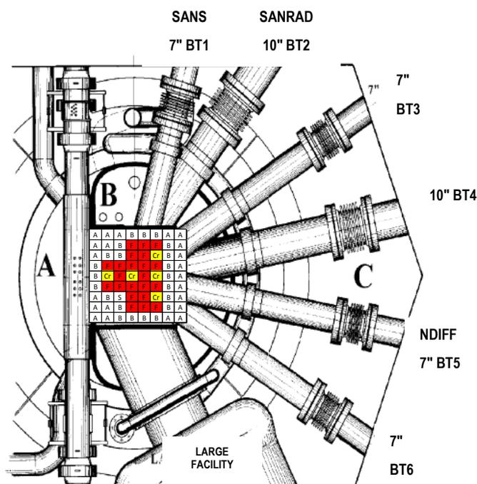
Figure 1: Top view layout of the SAFARI-1 reactor. Indicated positions refer to: A: Pool-side facility, B: In-core positions, and C: the radial beam lines.
