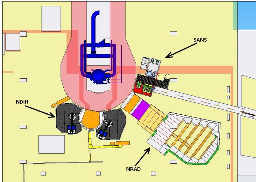
Figure 2: Top view layout of the beam line facilities in the SAFARI-1 reactor hall. The second phase of the SANS development will extend through the containment wall on the Eastern side of the reactor hall.
