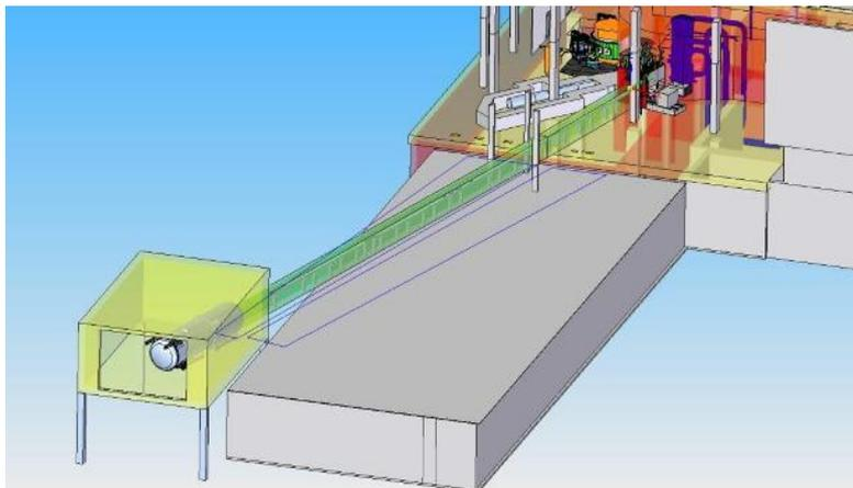
Figure 3: Artistic impression on SANS Phase 2 extending through the Eastern wall of SAFARI-1 building with curved neutron guide and doubled scattering chamber.
